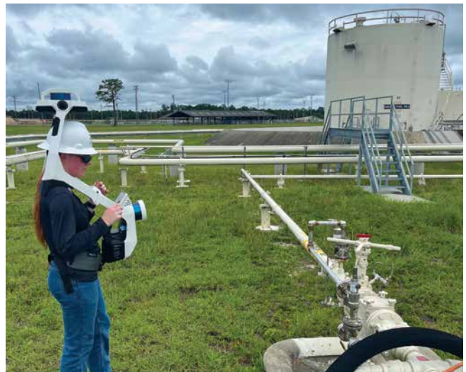
We have used 3D scanning to provide fuel system maintenance and minor repairs for over 8 years.
