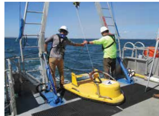
SUB-BOTTOM PROFILER DEPLOYMENT
